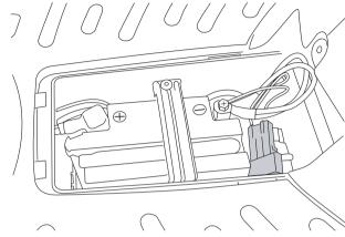
Find the faulty fuse by looking at the condition of its filament
