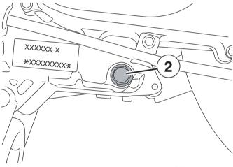
Remove the drainage cap and its seal (2) and allow the oil to drip into a recipient.
