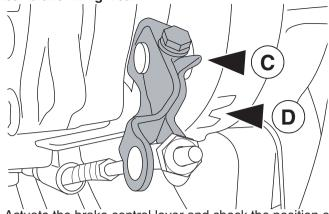
Actuate the brake control lever and check the position of the wear mark on the cam tierod (C) compared to the mark (D) on the engine housing.
