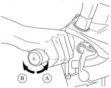
To accelerate, turn the throttle towards (A). To slow down, turn the throttle towards (B).
