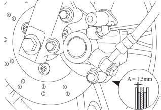
If one of the 2 brake pads is worn down to the minimum dimensions (A), the 2 brake pads must be changed.
