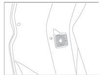
The utility hanger is located on the rear shield panel. It can be used to attach a maximum load of 2.5 kg.
