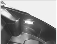
If a storage compartment is left open, the lighting automatically switches off after 4 minutes.
