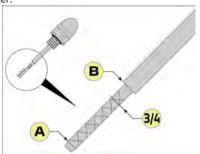
If the oil level is close to the minimum mark or lower, you are advised to immediately top up the level to 3/4 in small amounts using the oil recommended by the manufacturer.
