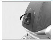
Located in front of the saddle this is used to hang a bag weighing not more than 2.5 kg.
