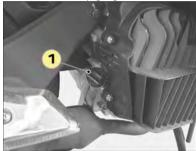
· Wipe the filler cap/gauge using a clean cloth and reinsert it into the filler hole without screwing it up.
