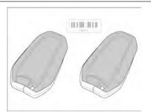
The Smart Key key is an electronic key which is recognised by the system within a radius of 1.5 meters and:
